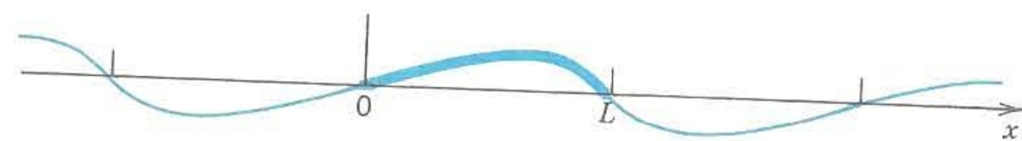
Fig. 254. Odd periodic extension of f(x)
