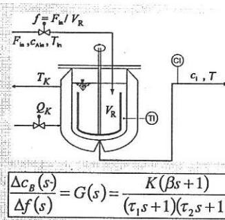
$$\begin{aligned} \frac{dc_A}{dt} &= \frac{F_{in}}{V_R} \cdot (c_{Ain} - c_A) - [k_1(T)c_A + k_3(T)c_A^2] \\ \frac{dc_B}{dt} &= \frac{F_{in}}{V_R} c_B + [k_1(T)c_A - k_2(T)c_B] \end{aligned}$$
