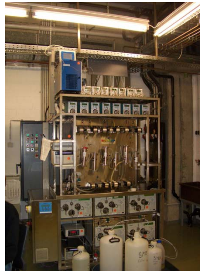
Novasep SMB plant, with reactors on top
