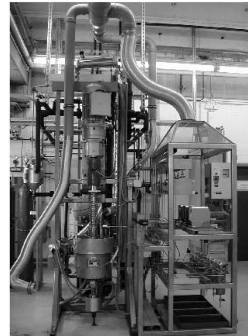
Pilot Plant 10l stainless steel reactor DCS controlled
