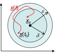
If the initial state  $\underline{x}(t_0)$  is sufficiently close to a stable equilibrium  $\underline{x}_s$ , then the state of the system stays close to  $\underline{x}_s$  for all times.
