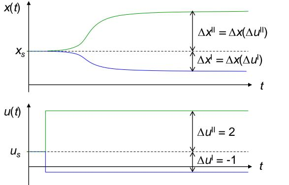
Check  $\Delta \underline{x}$  for different  $\Delta \underline{u}$  for the nonlinear system, e.g.:
