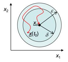
If more than one equilibrium exists, each stable equilibrium  $\underline{x}_s$  has a domain of attraction, i.e., the trajectories  $\underline{x}(t)$  that start inside the domain of attraction stay inside.
