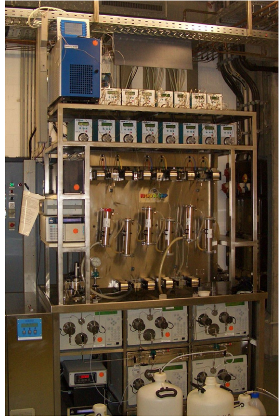
Fig. 8. Experimental SMB-plant with external reactors (in the heated bath on the top, left).
