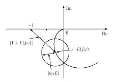
$$\begin{array}{lll} RS & \Leftrightarrow & |w_{l}L| < |1+L|, \quad \forall \omega \\ & & & \\ \left| \frac{w_{l}L}{1+L} \right| < 1, \ \forall \omega \quad \Leftrightarrow \quad \|w_{l}T\|_{\infty} < 1 \end{array}$$
