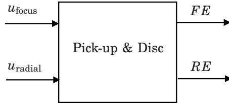
Figure 5.7 The pick-up head and disk seen as a two-input, two-output dynamical system.
