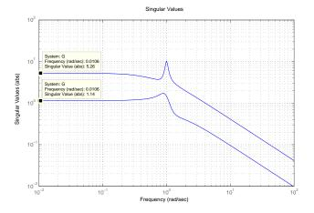
Figure: The singular values of the tranfer function matrix (prev slide). Note that G(0)=[2,4;03] which corresponds to M in the SVD-example above.  $\|G\|_{\infty}=10.3577.$
