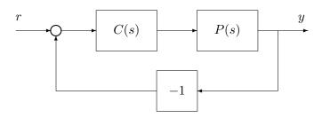
$$Y(s) = \underbrace{\frac{P(s)C(s)}{1 + P(s)C(s)}}_{T(s)} R(s)$$
