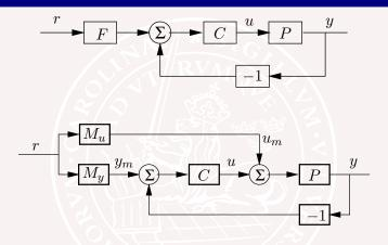
For linear systems all 2DOF configurations have the same properties. For the systems above we have
