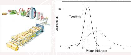
All paper production below the test limit is wasted. Good control allows for lower setpoint with the same waste. The average thickness is lower, which saves significant costs.
