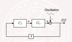
A model of how the disk oscillation affects the system. For example, if the oscillation offset at some point in time is +6.2 tracks, the DVD radial servo has to be at +6.2 tracks too to have zero RE.
