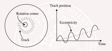
The disc is often a bit eccentric (i.e. not rotating around the track center). The resulting track position, which the Pick-Up-Head has to follow, is sinus-like.
