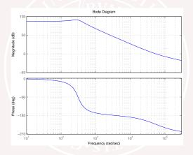
System identification made by sinusoidal excitation.
