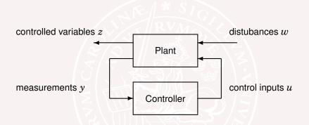
For a linear plant, minimize a quadratic function of the map from disturbance w to controlled variable z
