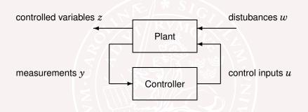
The objective is to find a controller that optimizes the transfer matrix  $G_{zw}(s)$  from disturbances w to controlled outputs z.
