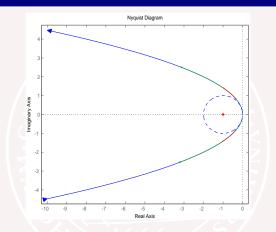
Notice that the distance from  $L(i\omega I - A)^{-1}B$  to -1 is never smaller than 1. This is always true(!) for linear quadratic optimal state feedback when  $Q_1 > 0$ ,  $Q_{12} = 0$  and  $Q_2 = \rho > 0$  is scalar. Hence the phase margin is at least 60°.
