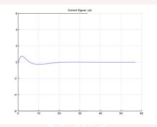
The step input stays within its amplitude bound  $|u(t)| \leq 6$ .
