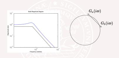
An lower bound  $|G(i\omega_i)|$  is a *non-convex* quadratic constraint. This should be avoided in optimization.
