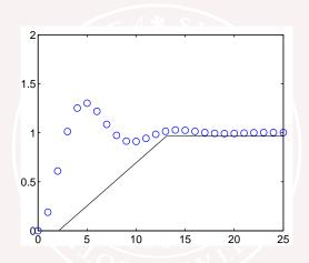
The step response depends linearly on  $Q_k$ , so every time  $t_k$  with a lower bound gives a linear constraint.
