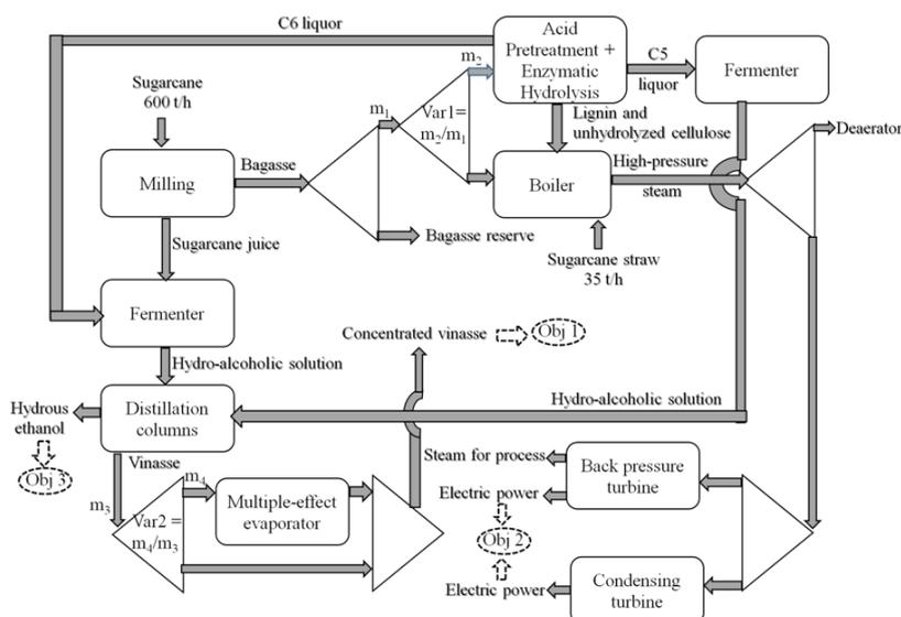
**Figure 2. Schematic representation of the process, with representation of studied objective functions and decision variables.**
